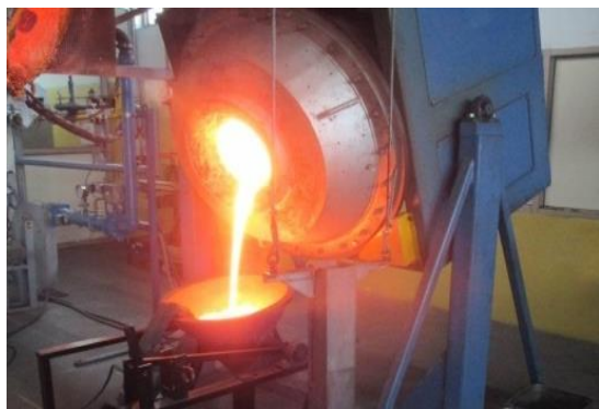
Fig. 5 Fire refined copper poured out from TBRF
