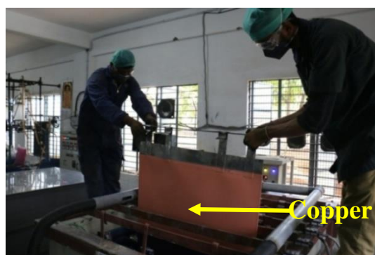
Fig.7 Electro refining of Copper
