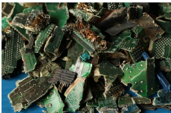
Fig.2. Depopulated, shredded PCBs
